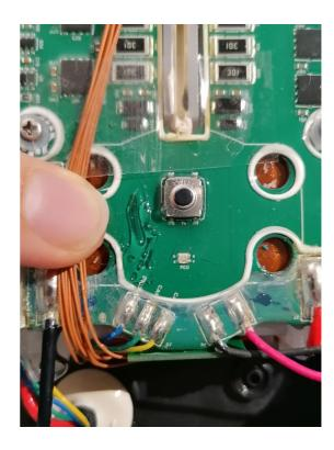
Once tidy, have a look at the expected result below and on the next page. Apply cyanoacrylate glue from the bottom, wait until cured. Re-execute these operations: partially remove duct tape  $\rightarrow$  glue  $\rightarrow$  wait.
