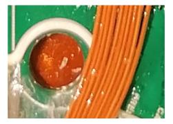
• Make sure the wires are located below the left and right neighboring conformal coating:
