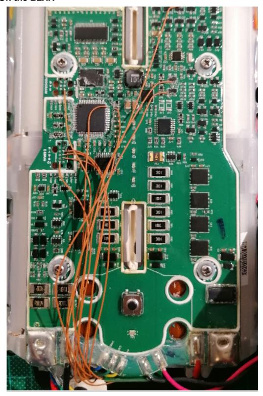
**Important:** Solder the wires following the order defined in table page 3 (from '-' to 'c'). Make sure they are not tangled. The next step will consist in testing and tidying the mess.
